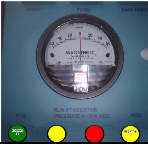
Prior to spraying, Technicians must set the Magnehelic Gauge to NEGATIVE Pressure between -0 and -10PA using the balance controls illustrated above.
