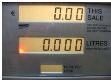
Fig1, Wayne dial face with Fault LED Note: On Tokheim Dial Face LED is separate at the left hand end of the litres display
