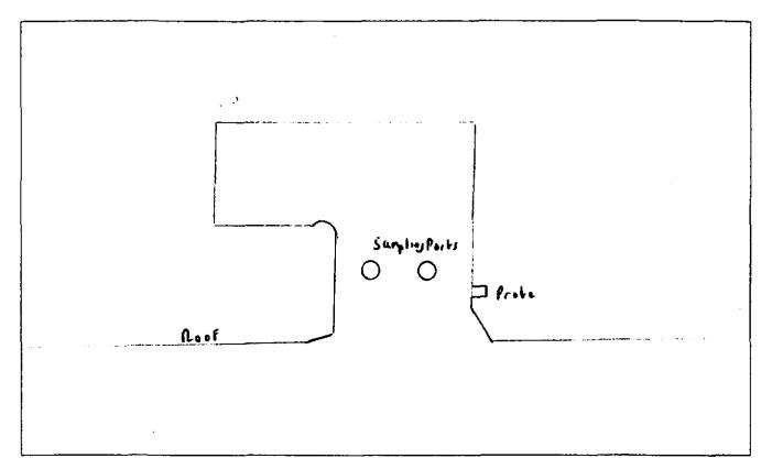
2) Section of duct at sample place and dimensions
