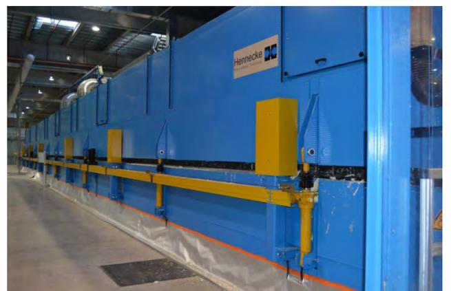
Substances mix at the pouring head – extraction of pentane fume to atmosphere
