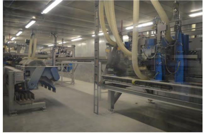
Solid blocks of insulation foam are cut to size in the knife section
