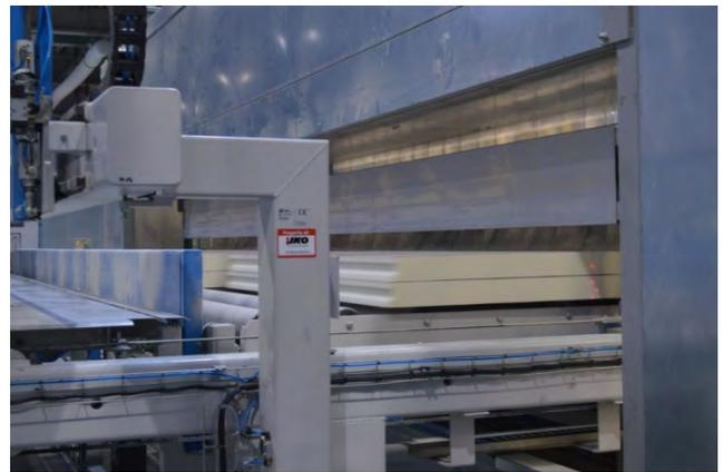
Solid blocks of insulation foam pass through stacked conveyor to cure fully
