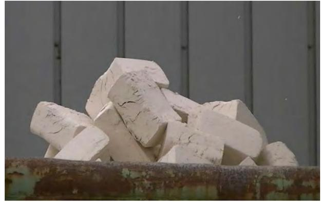
Dust from the cutting sections is processed through the briquette machine before storage in skips for disposal – it is anticipated that this will be sent for refused derived fuel as opposed to landfill
