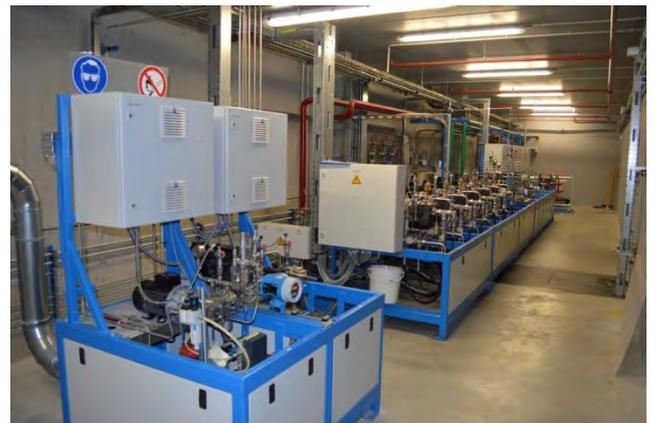
Chemicals are pumped to the machine along 'gas safe' colour coded lines and equipment, 'atex' approved equipment for pentane transfer
