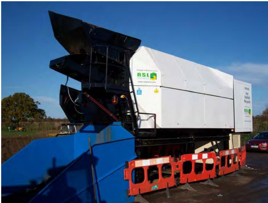
The Recycling Plant: The black funnel is where the old road planings are inserted into the drum mixer. The planings are then reheated and broken up.
