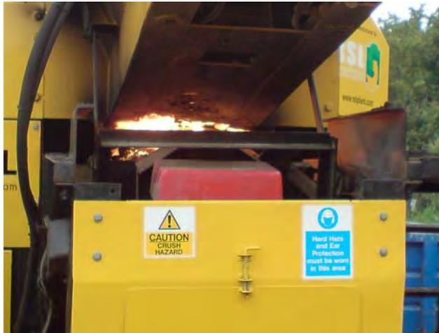
Fig. 3: View of rear of plant showing internal gas burners
