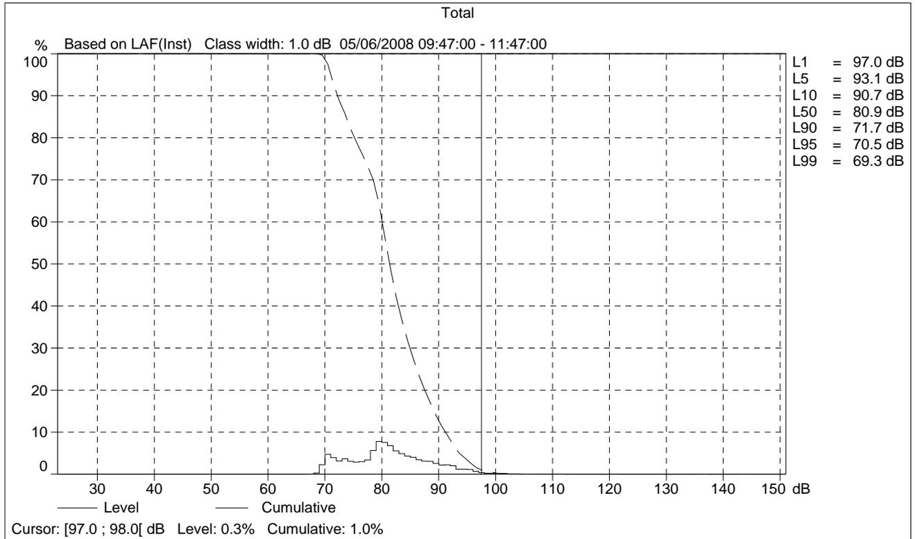
**NOISE DOSIMETRY: Asphalt Recycling Ltd**
