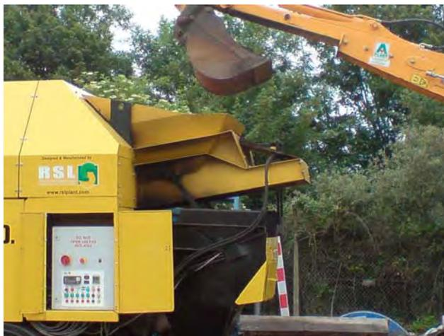
Fig. 2: Used material being loaded into recycling machine
