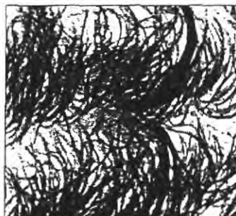
The filtering surface of the SUPERBAG 2000, enlarged 30 times.
