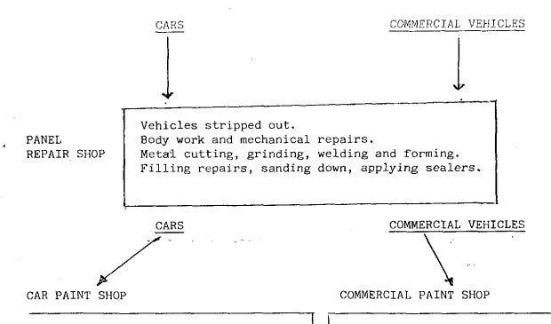
Preparing - sanding down etc. Priming and finish painting with I.C.I. 2 pack products in two proprietary low bake ovens.
