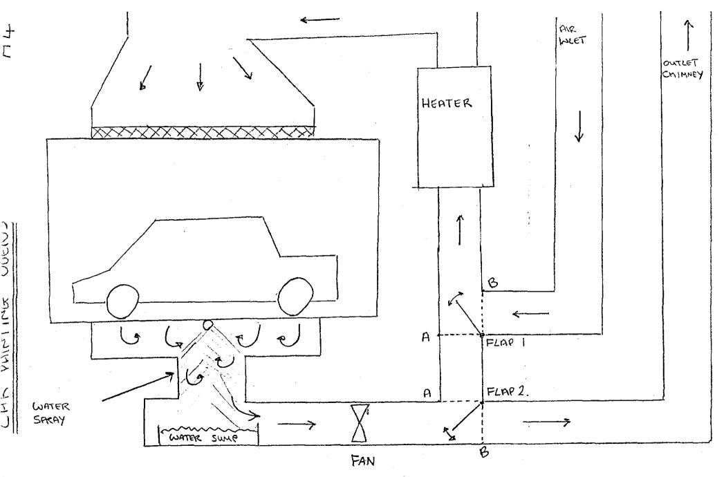
1. SPRAY CYCLE - FLARS 1+2 POSITION 'F'. AIR HEATTO, FILTYTED INTO SPRAY BOOTH, WATTER WASHED AND EMITTED FROM CHIMNEY
