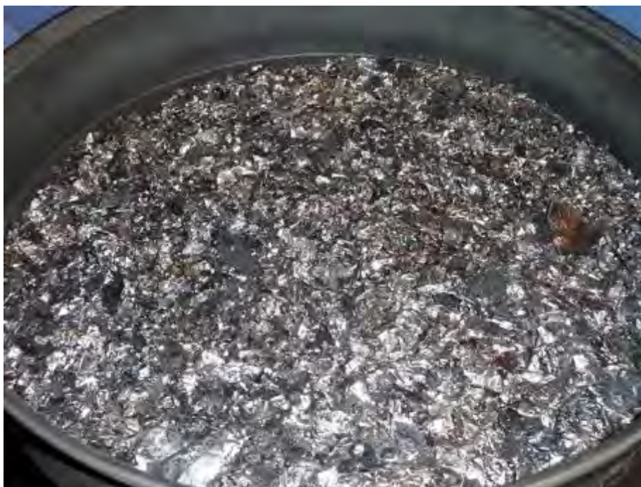
Figure 6: Photograph of the aluminium flakes produced (Test 5)
