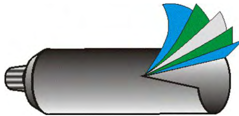
Figure 1: Different layers present in a typical toothpaste tube
