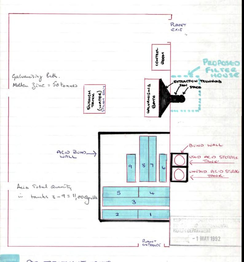
PRE-TREATMENT TANKS Y CAUSTIC CLEANGE TANK 3 WATER RINSE 3-9 HYDROCHERIC ACID TANKS
