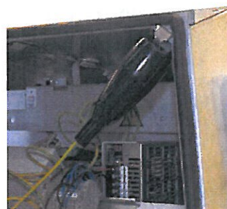
Figure 59 Connect the calibration kit ground cable.
