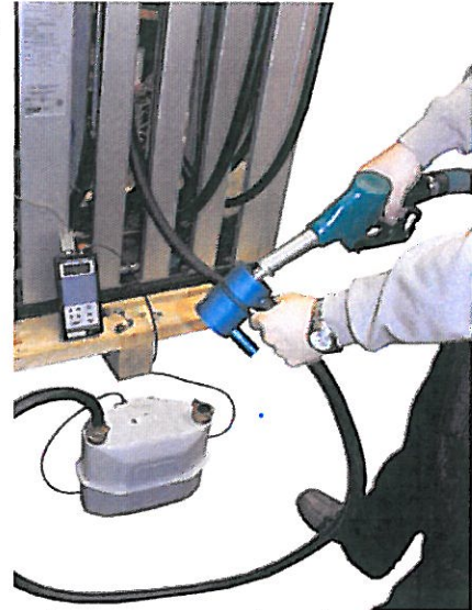
Figure 61 Connect the Bürkert meter to nozzle
